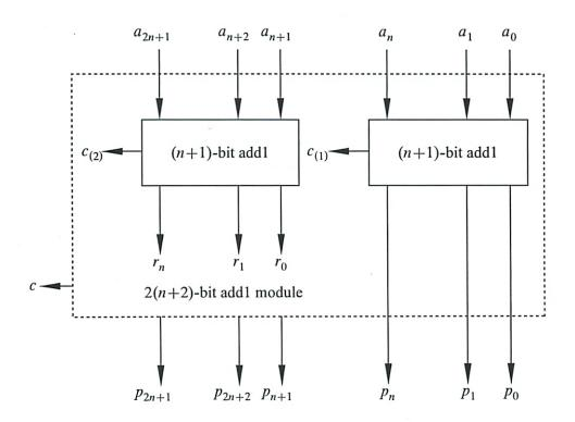
Figure 1 Structure of a Double-size Add1 Module.
